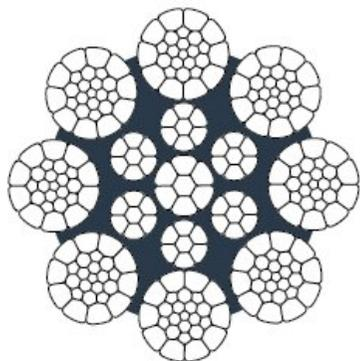
**Typical applications:** When rotation resistant ropes are not required (twin hoist systems with right and left ropes, small heights). Hoist for steel mill cranes, container cranes, floating cranes and boom hoist for deck cranes, luffing and mobile cranes, grab cranes.
